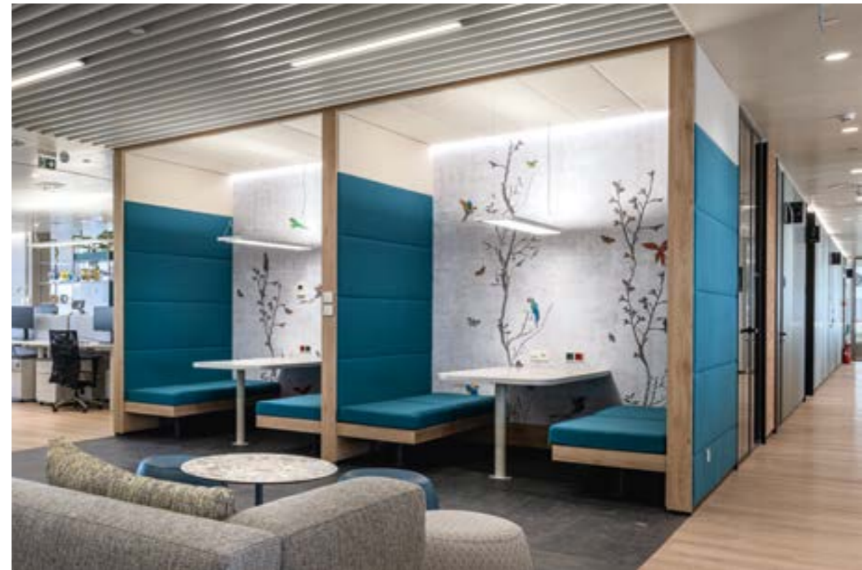
Vibrasto acoustic cladding on partitions and seats of acoustic alcoves in an open plan area of mobile network operator Cosmote's head office in Athens, Greece. Architects: Katerina Karanikou and Giorgos Stamatakis of A-team MELETI LTD. Nikos Kontopoulos of Calma Acoustics, 2023.
